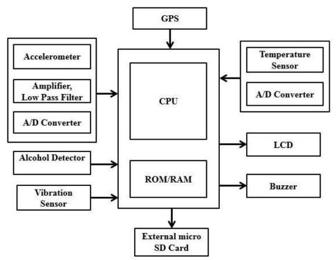
Fig- 3:Hardware Configuration Block Diagram
